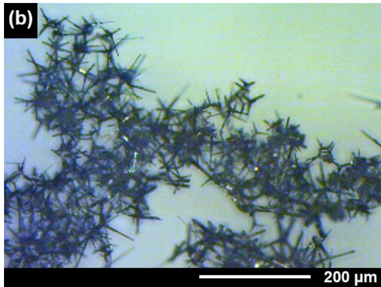
Interaction between many GaN/ZnO hollow tetrapods on water surface
