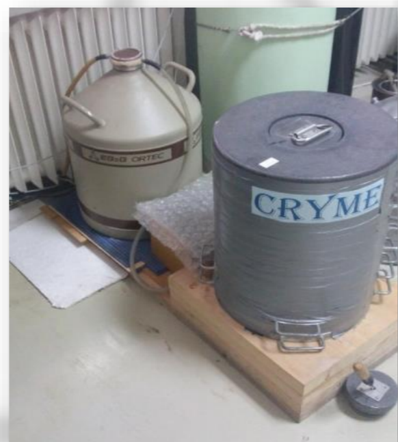
Fig. 2. ORTEC gamma spectrometry system for measuring radioactivity.
