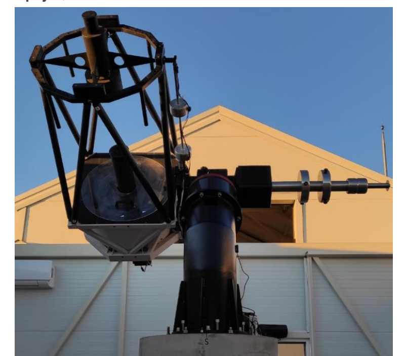
Fig.1c Telescope Nedeljković - 60 cm mirror
