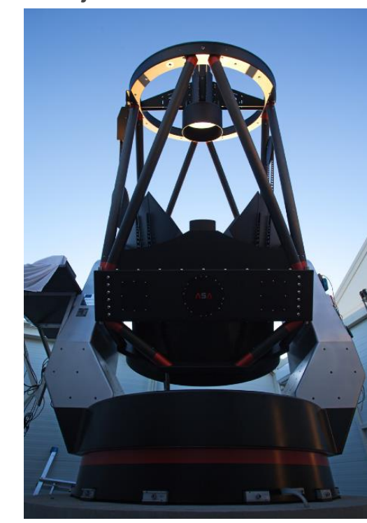
Fig.1b Telescope Milanković - 140 cm mirror
