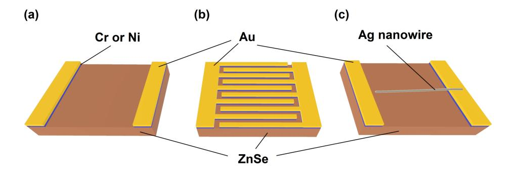
Fig. 1. Schematic structure of ZnSe-based metal-semiconductor-metal UV photodetector with different contacts design: (a) conventional contacts ; (b) interdigital contacts; (c) hybrid Ag-NW contacts
