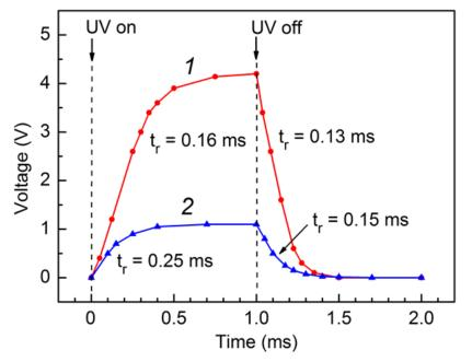
The response times are equal to 0.25 ms and 0.15 ms for a UV photodetector with conventional contacts, and are equal to 0.16 ms and 0.13 ms for a UV photodetector with interdigital contacts, respectively.
