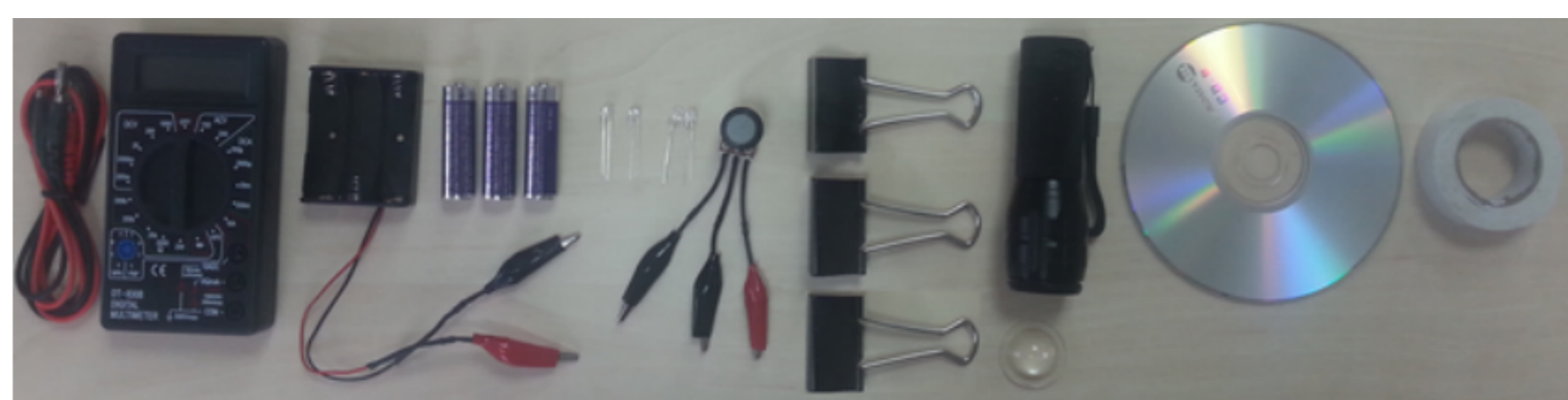
Figure 5: Details from the experimental set for measuring the Plank constant h: Wires ending with plug and crocodile clip, multimeter, battery holder and 3 batteries of 1.5 V, 4 LEDs, potentiometer with wires ending with crocodile clips, 3 binder clips, touch and its lens, Compact Disc (CD) double stick tape, photo-resistor, non transparent tube, plasticine, paper clip.
