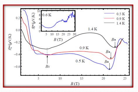
• The inset shows the interlayer magnetothermopower the organic conductor  $\alpha$ -(ET)<sub>2</sub>KHg(SCN)<sub>4</sub> at low temperature of 0.6 K
