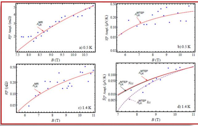
The amplitude  $A_{LK}$  of the first harmonic of the oscillations in the single band is given by  $A^{MR}{}_{LK} \sim R_T R_D R_S$  for MR and  $A^{MTEP}{}_{LK} \sim B^{-1/2} R_T R_D R_S$  for MTEP.  $R_T = (14.69m * T/B)/sinh(14.69m * T/B) - the temperature factor,$  $R_D = exp(-m_b T_D/B) - the Dingle$  $factor, <math>R_S = cos(gm_b/2m_e)$  is the spin factor.
