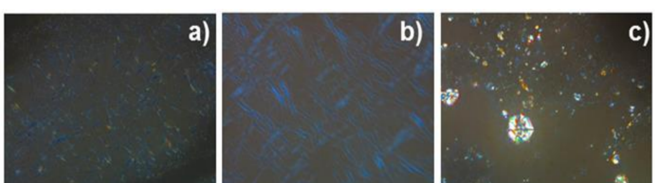
Fig.3. POM of nanocomposite (cross-polars, 40x, heating rate 5°C/min: a) at room temperature, the sample is as prepared; b) heating, at 92°C - the fibres melt; c) at subsequent cooling (0.2°C/min) - mixed texture consisting of fibre-like network and spherical coloured domains.
