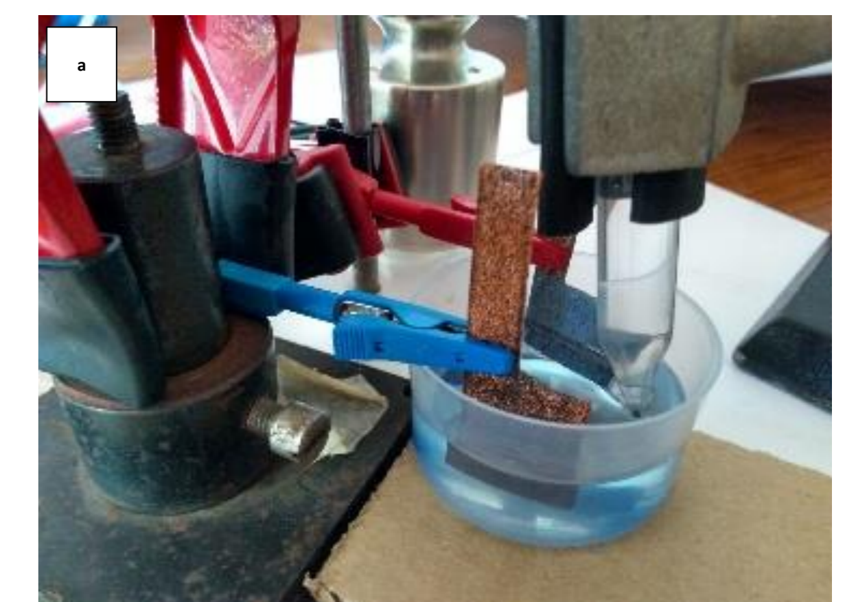
Bio-logic SP-200 potentiostat/galvanostat & three-electrode configuration experimental setup
