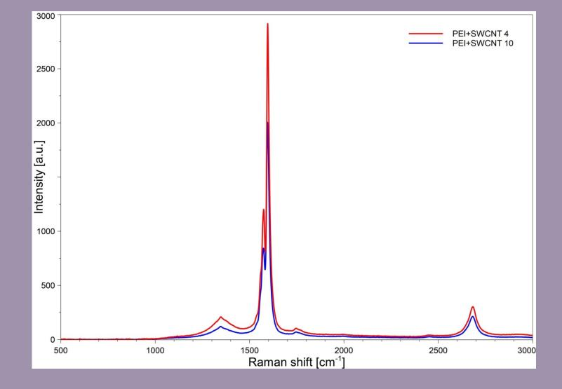
In a SWCNT, the G band splits into G<sup>+</sup> and G<sup>-</sup> peaks due to the strain effect, which is related
