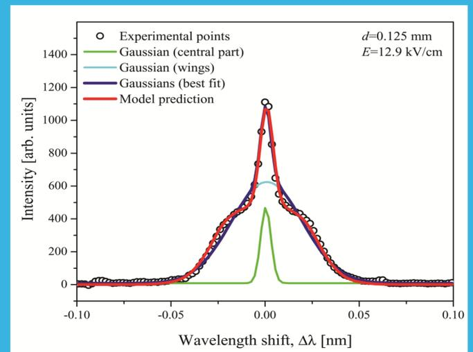
**Fig. 3.** The comparison between the prediction of the iterative kinetic model [3] with the best fit obtained by the model function (1) of the Ne II 371.308 nm line profile.
