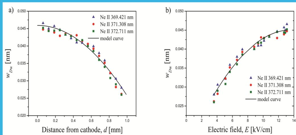
**Fig. 4.** (a) Symbols show the FWHM of the Doppler profile  $w_{Dw}$  of line wings against distance from the cathode,  $d$ , and the full line shows the phenomenological model curve (2) which predicts the average variation of  $w_{Dw}$  with  $d$  for the three Ne II lines recorded side-on. (b) The same as in (a), but for the correlation (3) between  $w_{Dw}$  and the strength of electric field  $E$ .
