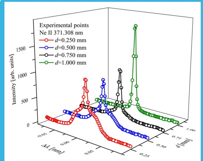
**Fig. 2.** 3D plot of the spectral profiles of Ne II 371.308 nm line recorded side-on at four distances  $d$  from the cathode. Line intensity is shown against the wavelength shift  $\Delta\lambda = \lambda - \lambda_0$  from the central wavelength  $\lambda_0 = 371.308$  nm.
