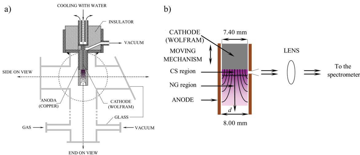
**Fig. 1.** Schematic drawing of modified Grimm glow discharge source [1, 2]. b) A magnified view of the encircled part from a).
