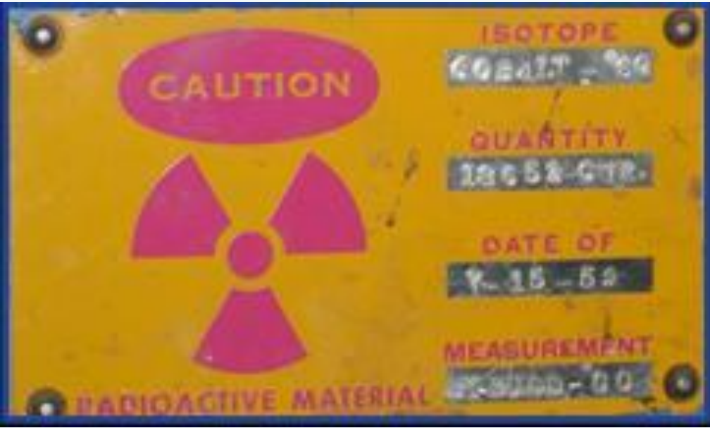
Figure Nr.1 Example of labels on the radioactive sources or devices
