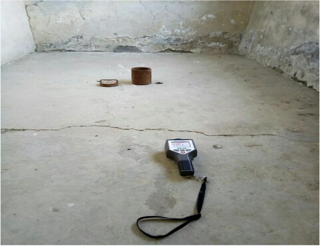
Figure Nr.2 Measurement of dose rate at 1 m distance.
