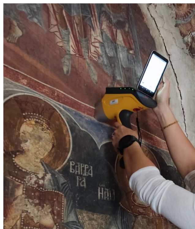
Figure 2: Portable X-ray fluorescence (XRF) Explorer 5000 device.
