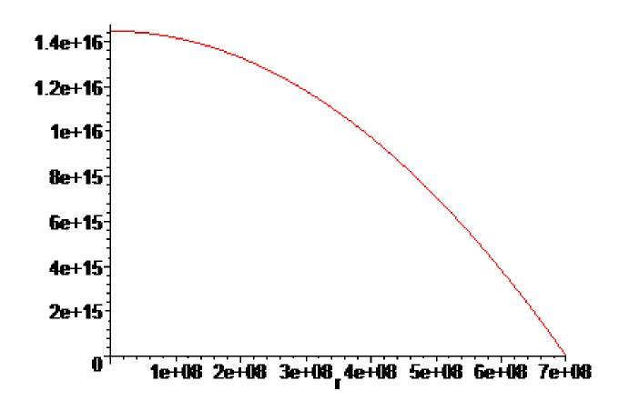
Central pressure P(0.01Pa) of star Sun in function of radius r(m). R=700000km,  $\rho$ =1500kg/  $m^3$
